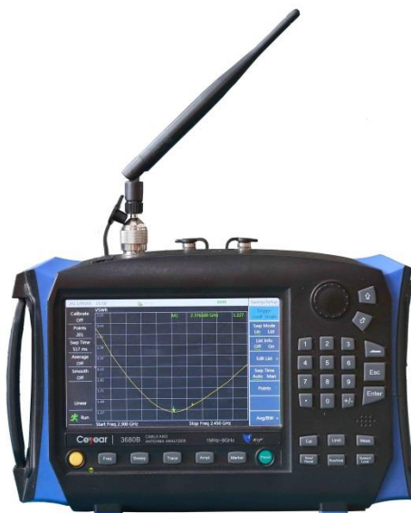
Antenna return loss/VSWR measurement
